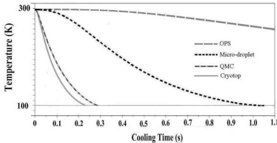
Figure 2. The predicted temperature at the warmest point of the oocyte in four different vitrification systems immersed in liquid nitrogen for an external heat transfer coefficient  $h = 2000 \text{ W/m}^2 \cdot \text{K}$ .
