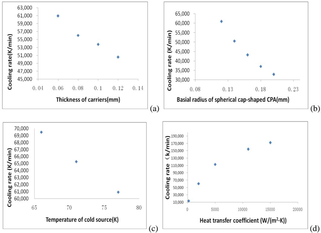
Figure 3. Effect of thicknesses of carrier (a), basal radius of spherical cap-shaped CPA (b), temperature of cold source (c), and heat transfer coefficient (d) on the cooling rate in Cryotop.
