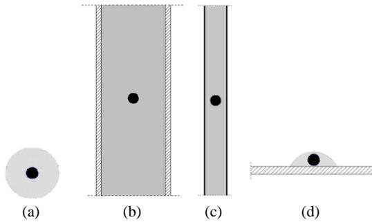
Figure 1. Geometry of four physical models used for numerical simulation: (a) the Micro-droplet model, (b) the OPS model, (c) the QMC model, and (d) the Cryotop model. The black dots represent the oocyte, whereas the gray domain stands for CPA solution. The domains with diagonal stripes in (b) and (d) stand for PVC and black line in (c) stands for quartz.
