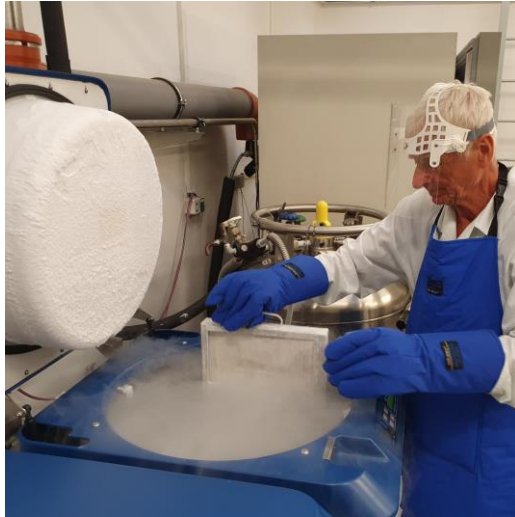
Figure 1. The cryostorage frame with inserted metal cassettes containing cryopreserved vascular grafts in the liquid nitrogen storage vessel.
