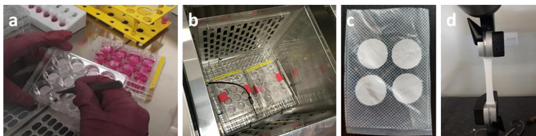
Figure 3. "In-air" cryopreservation workflow adapted for electrospun stem cell-seeded scaffolds: (a) cell seeding onto scaffolds; (b) in-plate cryopreservation; (c) cryopreservation in cryobags; (d) mechanical testing following cryopreservation.
